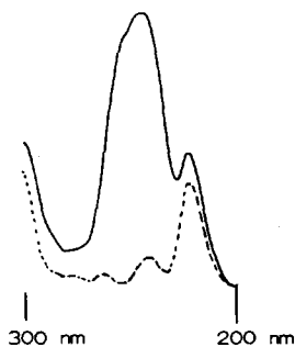
Fig. 5. Fluorescence excitation spectrum for carazolol (—) and the eluent (.....) taken by a stop flow scan at emission wavelength 351 nm; scan speed 1.5 nm/s; paper advance 1 mm/s. The HPLC conditions as described in Materials and methods.
